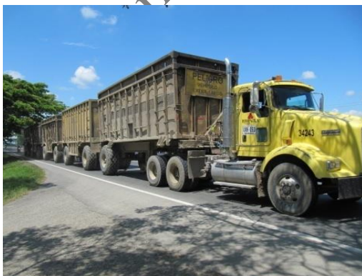
Romeu e Julieta: five axle combination including a truck and a trailer
