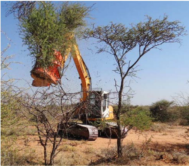
Mechanised bush harvesting using a customised excavator with hydraulic shear (Ohlthaver & List).
